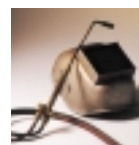
Figure 1 The use of a controlled mixture of oxygen and acetylene provides the best conditions and very high temperatures necessary for cutting or welding metal. Note the hose boxes leading to the torch.
