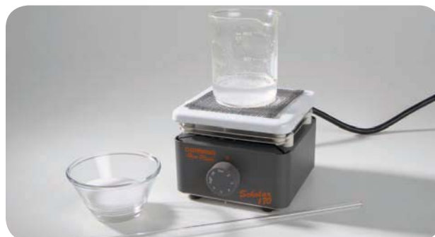
Figure 2 One technique for removing water from a mixture
